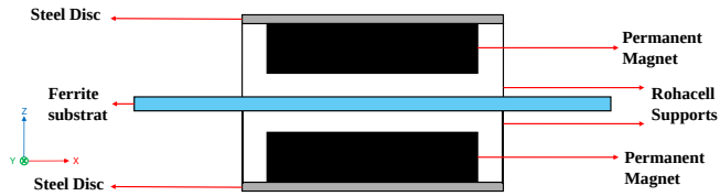
Fig. 7. Magnetostatic simulation configuration.
