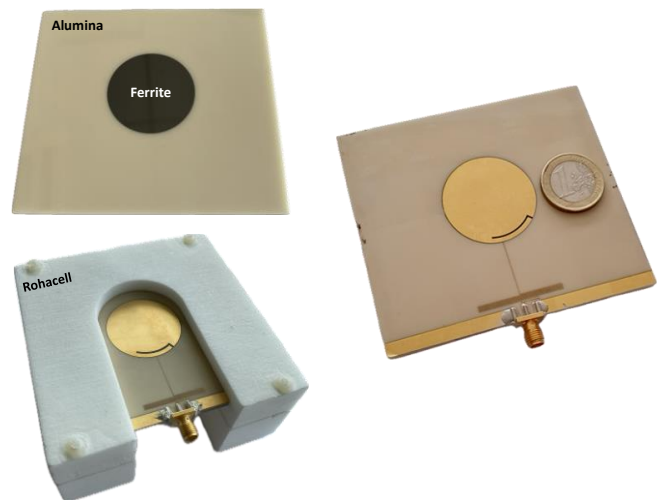
Fig. 18. The bare ferrite and alumina substrate, the fabricated antenna after metallization and laser etching and the antenna mounted inside the Rohacell support.
