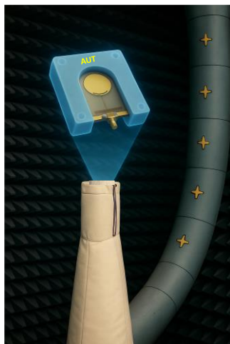
Fig. 19. SG 24 Stargate measurement setup used for the characterization of the fabricated antenna (antenna under test – AUT).
